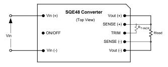
Fig. C: Configuration for increasing output voltage.
