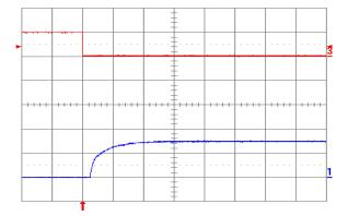
**Fig. 1.5V.8:** Turn-on transient at full rated load current (resistive) plus 10,000  $\mu$ F at Vin = 48 V, triggered via ON/OFF pin. Top trace: ON/OFF signal (5 V/div.). Bottom trace: Output voltage (1 V/div.). Time scale: 2 ms/div.
