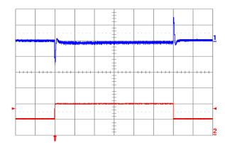
Fig. 1.8V.10: Output voltage response to load current stepchange (10 A - 20 A - 10 A) at Vin = 48 V. Top trace: output voltage (100 mV/div.). Bottom trace: load current (10 A/div.). Current slew rate: 5 A/µs. Co = 470 µF POS + 1 µF ceramic. Time scale: 0.2 ms/div.
