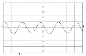
**Fig. 3.3V.11:** Output voltage ripple (20 mV/div.) at full rated load current into a resistive load with Co = 10  $\mu$ F tantalum + 1  $\mu$ F ceramic and Vin = 48 V. Time scale: 1  $\mu$ s/div..
