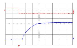
**Fig. 3.3V.8:** Turn-on transient at full rated load current (resistive) plus 10,000  $\mu$ F at Vin = 48 V, triggered via ON/OFF pin. Top trace: ON/OFF signal (5 V/div.). Bottom trace: Output voltage (1 V/div.). Time scale: 1 ms/div.
