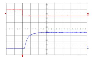
**Fig. 2.5V.8:** Turn-on transient at full rated load current (resistive) plus 10,000  $\mu$ F at Vin = 48 V, triggered via ON/OFF pin. Top trace: ON/OFF signal (5 V/div.). Bottom trace: Output voltage (1 V/div.). Time scale: 2 ms/div.
