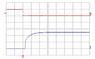
**Fig. 2.5V.7:** Turn-on transient at full rated load current (resistive) with no output capacitor at Vin = 48 V, triggered via ON/OFF pin. Top trace: ON/OFF signal (5 V/div.). Bottom trace: Output voltage (1 V/div.). Time scale: 2 ms/div.
