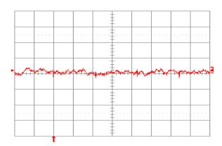
**Fig. 1.5V.14:** Input reflected-ripple current,  $i_s$  (10 mA/div.), measured through 10  $\mu$ H at the source at full rated load current and Vin = 48 V. Refer to Fig. 1.5V.12 for test setup. Time scale: 1  $\mu$ s/div.
