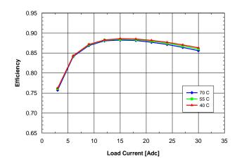
**Fig. 1.8V.4:** Efficiency vs. load current and ambient temperature for SQE48T30018 converter mounted vertically with Vin = 48 V and air flowing from pin 3 to pin 1 at a rate of 200 LFM (1.0 m/s).
