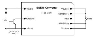
Fig. A: Circuit configuration for ON/OFF function.
