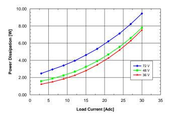
**Fig. 1.5V.5:** Power dissipation vs. load current and input voltage for SQE48T30015 converter mounted vertically with air flowing from pin 3 to pin 1 at a rate of 300 LFM (1.5 m/s) and Ta = 25 °C.
