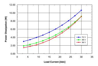
**Fig. 2.5V.5:** Power dissipation vs. load current and input voltage for SQE48T30025 converter mounted vertically with air flowing from pin 3 to pin 1 at a rate of 300 LFM (1.5 m/s) and Ta = 25  $^{\circ}$ C.
