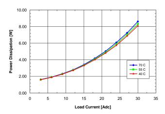
**Fig. 1.5V.6:** Power dissipation vs. load current and ambient temperature for SQE48T30015 converter mounted vertically with Vin = 48 V and air flowing from pin 3 to pin 1 at a rate of 200 LFM (1.0 m/s).
