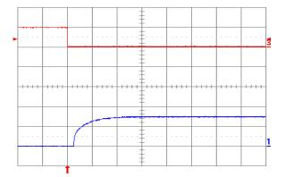
**Fig. 1.5V.7:** Turn-on transient at full rated load current (resistive) with no output capacitor at Vin = 48 V, triggered via ON/OFF pin. Top trace: ON/OFF signal (5 V/div.). Bottom trace: Output voltage (1 V/div.). Time scale: 2 ms/div.
