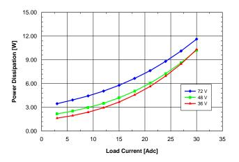
Fig. 3.3V.5: Power dissipation vs. load current and input voltage for SQE48T30033 converter mounted vertically with air flowing from pin 3 to pin 1 at a rate of 300 LFM (1.5 m/s) and Ta = 25  $^{\circ}$ C.
