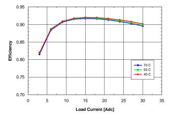
**Fig. 3.3V.4:** Efficiency vs. load current and ambient temperature for SQE48T30033 converter mounted vertically with Vin = 48 V and air flowing from pin 3 to pin 1 at a rate of 200 LFM (1.0 m/s).
