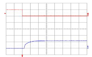
**Fig. 1.2V.8:** Turn-on transient at full rated load current (resistive) plus 10,000  $\mu$ F at Vin = 48 V, triggered via ON/OFF pin. Top trace: ON/OFF signal (5 V/div.). Bottom trace: Output voltage (1 V/div.). Time scale: 2 ms/div.
