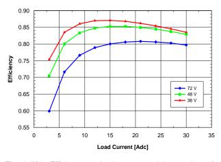
**Fig. 1.2V.3:** Efficiency vs. load current and input voltage for SQE48T30012 converter mounted vertically with air flowing from pin 3 to pin 1 at a rate of 300 LFM (1.5 m/s) and Ta = 25 °C.
