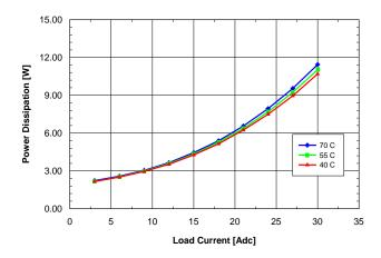
Fig. 3.3V.6: Power dissipation vs. load current and ambient temperature for SQE48T30033 converter mounted vertically with Vin = 48 V and air flowing from pin 3 to pin 1 at a rate of 200 LFM (1.0 m/s).
