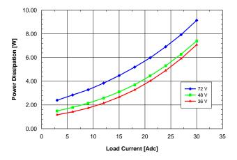
Fig. 1.2V.5: Power dissipation vs. load current and input voltage for SQE48T30012 converter mounted vertically with air flowing from pin 3 to pin 1 at a rate of 300 LFM (1.5 m/s) and Ta = 25  $^{\circ}$ C.
