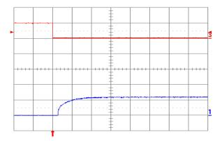
**Fig. 1.2V.7:** Turn-on transient at full rated load current (resistive) with no output capacitor at Vin = 48 V, triggered via ON/OFF pin. Top trace: ON/OFF signal (5 V/div.). Bottom trace: Output voltage (1 V/div.). Time scale: 2 ms/div.
