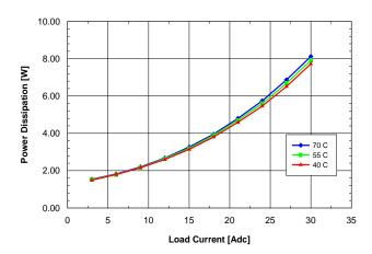
**Fig. 1.2V.6:** Power dissipation vs. load current and ambient temperature for SQE48T30012 converter mounted vertically with Vin = 48 V and air flowing from pin 3 to pin 1 at a rate of 200 LFM (1.0 m/s).
