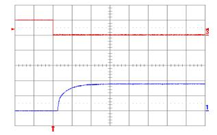
**Fig. 1.8V.8:** Turn-on transient at full rated load current (resistive) plus 10,000  $\mu$ F at Vin = 48 V, triggered via ON/OFF pin. Top trace: ON/OFF signal (5 V/div.). Bottom trace: Output voltage (1 V/div.). Time scale: 2 ms/div.
