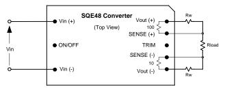
Fig. B: Remote sense circuit configuration.
