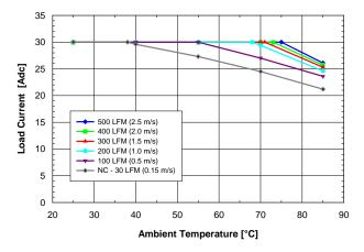
**Fig. 1.8V.2:** Available load current vs. ambient air temperature and airflow rates for SQE48T30018 converter mounted horizontally with air flowing from pin 3 to pin 1, MOSFET temperature  $\leq$  120 °C, Vin = 48 V.
