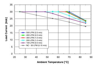
**Fig. 2.5V.2:** Available load current vs. ambient air temperature and airflow rates for SQE48T30025 converter mounted horizontally with air flowing from pin 3 to pin 1, MOSFET temperature  $\leq$  120 °C, Vin = 48 V.
