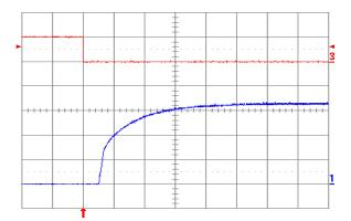
**Fig. 3.3V.7:** Turn-on transient at full rated load current (resistive) with no output capacitor at Vin = 48 V, triggered via ON/OFF pin. Top trace: ON/OFF signal (5 V/div.). Bottom trace: Output voltage (1 V/div.). Time scale: 1 ms/div.
