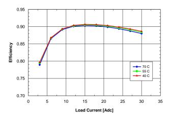
Fig. 2.5V.4: Efficiency vs. load current and ambient temperature for SQE48T30025 converter mounted vertically with Vin = 48 V and air flowing from pin 3 to pin 1 at a rate of 200 LFM (1.0 m/s).
