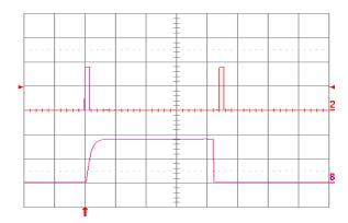
**Fig. 2.5V.16:** Load current (top trace, 20 A/div., 50 ms/div.) into a 10 mΩ short circuit during restart, at Vin = 48 V. Bottom trace (20 A/div., 2 ms/div.) is an expansion of the on-time portion of the top trace.
