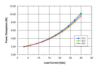
**Fig. 2.5V.6:** Power dissipation vs. load current and ambient temperature for SQE48T30025 converter mounted vertically with Vin = 48 V and air flowing from pin 3 to pin 1 at a rate of 200 LFM (1.0 m/s).
