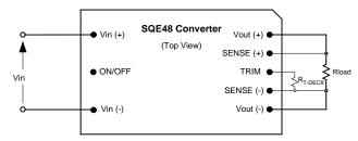
Fig. D: Configuration for decreasing output voltage.
