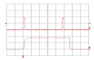
**Fig. 1.8V.16:** Load current (top trace, 20 A/div., 50 ms/div.) into a 10 mΩ short circuit during restart, at Vin = 48 V. Bottom trace (20 A/div., 2 ms/div.) is an expansion of the on-time portion of the top trace.
