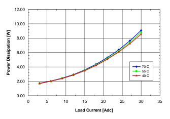
**Fig. 1.8V.6:** Power dissipation vs. load current and ambient temperature for SQE48T30018 converter mounted vertically with Vin = 48 V and air flowing from pin 3 to pin 1 at a rate of 200 LFM (1.0 m/s).
